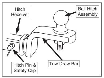
**Figure 2.** Tow draw bar installed in "upper" configuration.
